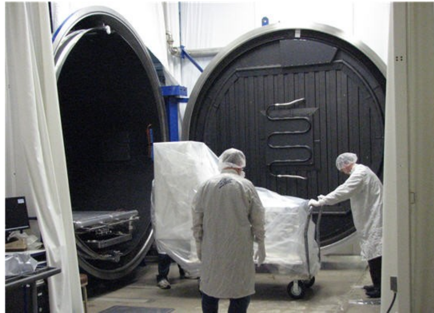
Loading OLI into Space Vacuum Simulation Chamber
